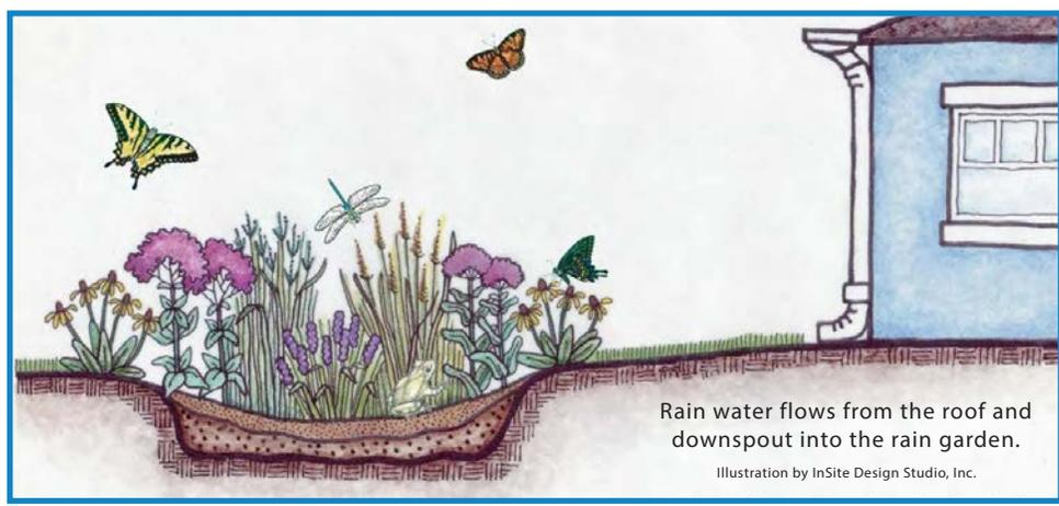
Rain water flows from the roof and downspout into the rain garden.
